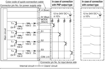
Symbols...D<sub>1</sub> to D<sub>8</sub>: Reverse supply polarity protection diode Tr1 to Tr4: PNP input transistor, Tr5 to Tr8: NPN input transistor
