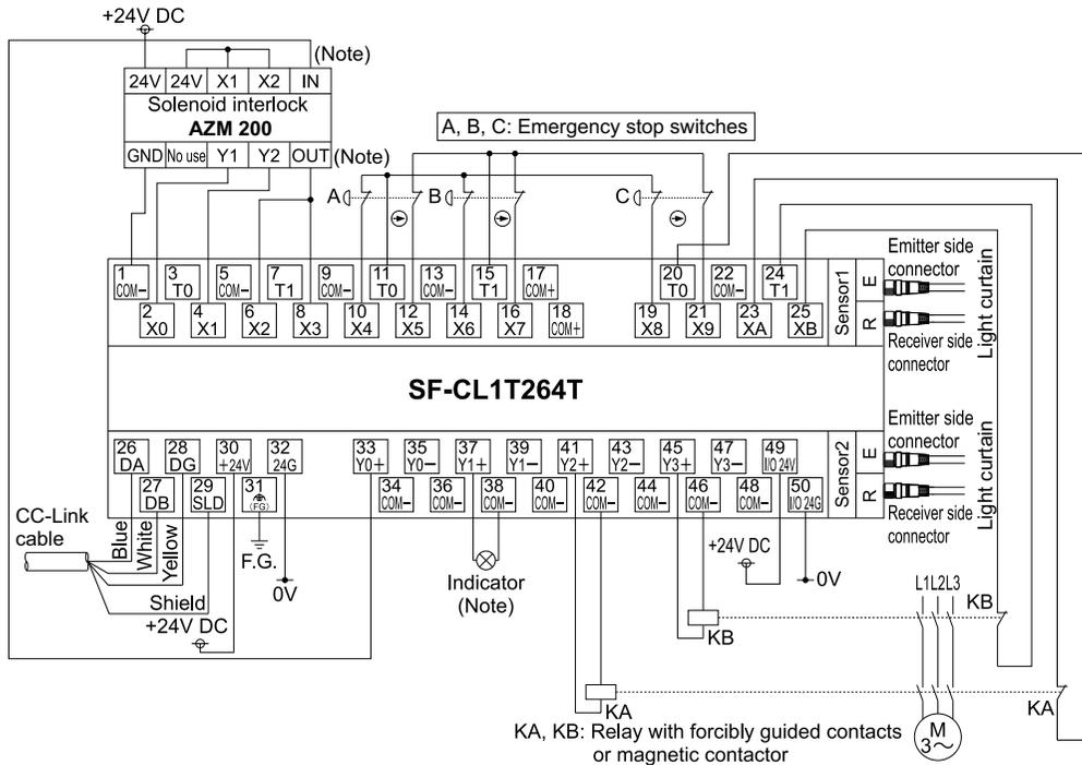
Note: Solenoid input (IN), diagnostic output (OUT) and the indicator of Solenoid interlock **AZM 200** can be connected to either this product or standard remote I/O unit.
